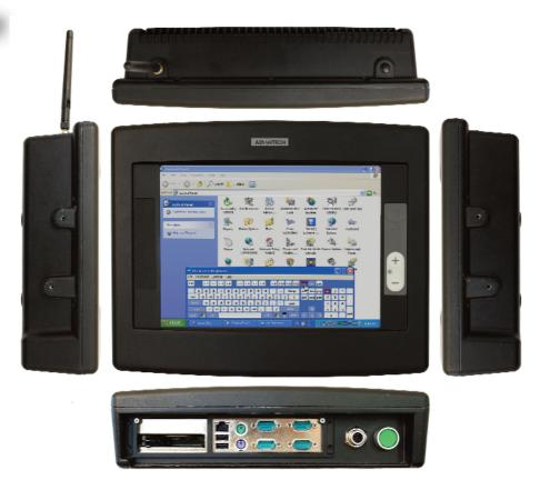
ing angle is 110 degrees, which is still sufficient in a vehicle mount. Advantech rates the LCD's mean time between failure at 50,000 hours. If the display were on 24 hours per day every day, that'd still be 5.7 years. The backlight is rated to have the same lifespan. Unlike Tablet PCs that often have a variety of hardware controls along the edge of the display, the TREK-775 has just one. You can increase and decrease screen brightness via two large integrated buttons.
