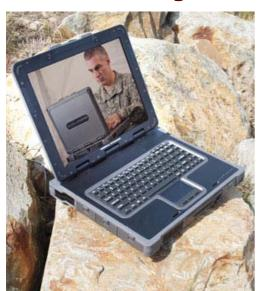
The Tadpole Topaz by General Dynamics is a rugged 12-pound notebook computer designed to provide functionality and performance that exceeds what is commonly available in the mobile computing space. Yet, its approach of using COTS ("commercial-of-the-shelf") technology and components results in a high-performance device that's substantially more affordable than what hardware specifically designed within military projects would cost.
