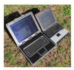
less blueish than what the camera captured, but the images accurately depict the difference in glare, reflection and contrast between the older model's display and the Topaz DynaVue screen.
