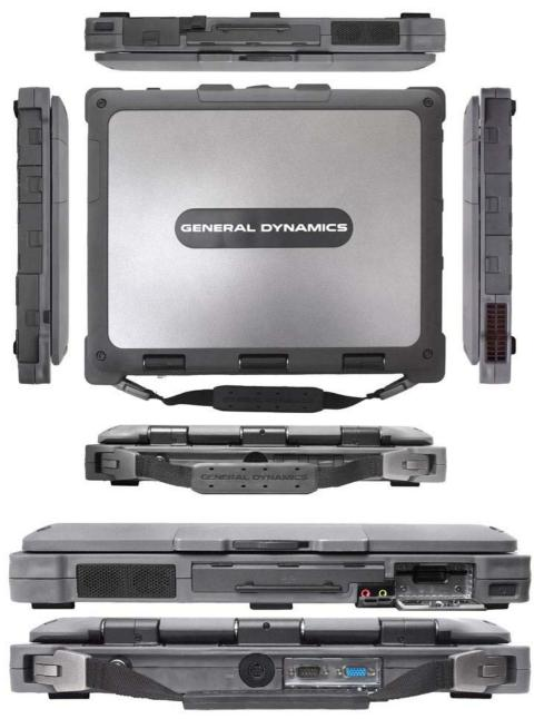
opening for the dual PC Card Type II slots (or one of the thicker Type III variety), and then the battery. Since the USB ports are fairly deeply recessed, USB keys may need an adapter cable to connect.
