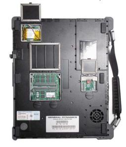
pact enclosure. Six rubber blocks serve as feet to create some air space underneath the unit. If it's sitting on carpeting or any other surface that obstructs proper airflow, you can instantly hear that in the pitch of the fan.
