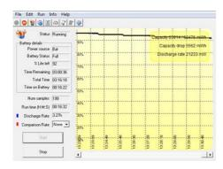
The Topaz, too, has a big battery, and that's because the machine needs it. Power consumption never dropped below 20 watts (the GD6000 used as little as 14.5 watts), and that's with WiFi off, the screen fairly dark, and the machine idling. At that rate, the battery would theoretically last about 3.5 hours. In real life continuous use, it's probably less.
