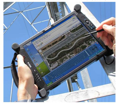
five-way navigation diamond that also doubles for brightness and volume control duty, a display rotation key, a WiFi/Bluetooth switch, a function hotkey, an ESC key, and the power button. The unit comes with a nicely designed stylus, 5.25 inches long, that can be tethered so it won't get lost, and has a secure garage on the backside of the computer.
