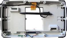
I/O is concentrated on either side of the motherboard. On one side, the connectors are soldered onto the motherboard. On the other they are on a separate daughterboard that contained a USB port and a DB-9 serial port. This design lends itself to easy customization, i.e. the Algiz could easily be configured with different daughterboards. The connectors on the daughterboard are sealed and form a second barrier should the primary barrier (the rubber/plastic plugs) be left open or leaking.
