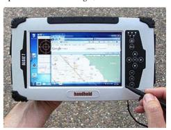
The outdoor-viewable 7-inch resistive touch screen display is large enough for real work and offers netbook-class 1024 x 600 pixel resolution. The screen is bright and crisp, resistant to smudges and fingerprints, and controls glare and reflections well. We'd like to see a wider vertical viewing angle and a dual-input option, either resistive/electromagnetic, or electromagnetic/capacitive.
