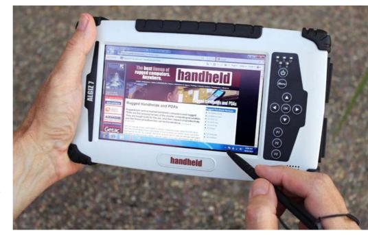
port, audio in and out jacks, a camera, and a multi-IO port for the optional cradle. Of the unit's four PCIe slots, one or more are available for expansion, and there are two SIM card slots. The outdoor-viewable display with its resistive touch screen measures just 7 inches diagonally, but has the same  $1024 \times 600$  pixel resolution used in tens of millions of netbooks.
