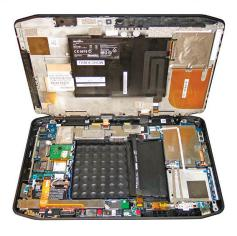
Sealing between the two halves of the housing is via a soft plastic sleeve that fits around the entire top half perimeter, and then forms a seal against the slightly bevelled inside perimeter of the bottom half once the two halves are compressed together.
