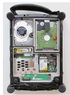
well designed, and very sturdy. Nothing rattles around and nothing is loose. This is as it should be in a rugged computer. In the picture to the left, you can see a number of expansion modules. There are two PCI Express slots, one of them taken up by an Intel
