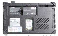
There are two removable covers on the backside of the RUGGEDBOOK SR820 (both removed in the picture above). One covers the battery and expansion slots, the other the optional WWAN module.
