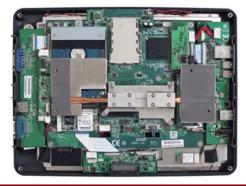
of separating the motherboard from interface boards allows the company to quickly and easily customize a machine for client applications without having to redesign the motherboard itself.
