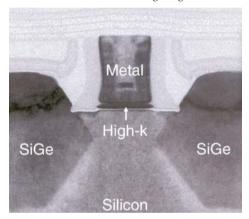
smaller, the conventional silicon dioxide gate materials began reaching their physical limits. This manifested itself in current leakage problems that resulted in high power consumption and reduced reliability. Searching for a way to solve that problem, it was found that high-k dielectric, or insulator, materials virtually eliminated these leakage problems.
