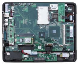
are known as the "Menlow" platform. The processor has about 47 million transistors, which is more than the Pentium 4 had. The chipset — which supports PCI-Express, SDIO, DDR2, LVDS, ATA 100, LPC and more — uses about 2.3 watts, which means total CPU and chipset consumption isn't even 5 watts. And the chipset even has hardware support for H.264 and other HD decoding. However, as the combo is targeted for internet devices, there is PATA but no SATA support.
