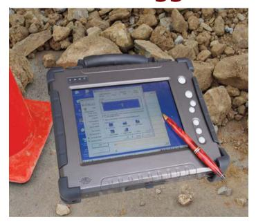
inmate's line of rugged Tablet PCs includes a variety of screen sizes, display technologies, and processor architectures. All share sturdy magnesium-aluminum housings and a basic, no-nonsense approach to tackling computing in the field under tough environmental settings. The I980 Series is built on the Intel Atom Z530 processor and thus represents one of the first rugged platforms to use this compact and highly owerefficient processor that offers unparalleled performance per watt.
