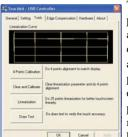
Touchkit control panel provides adjustment and optimization for accurate touch performance and ease of use. The panel is quite elaborate. You can set linearization either
