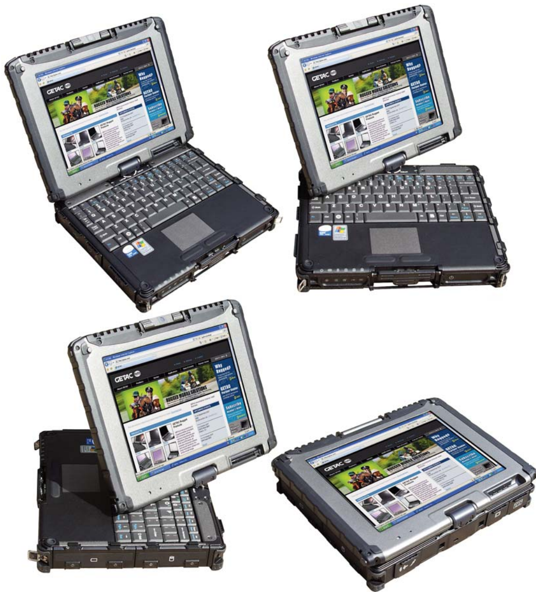
Above: The rugged GETAC V100 converts from notebook to Tablet PC slate.
