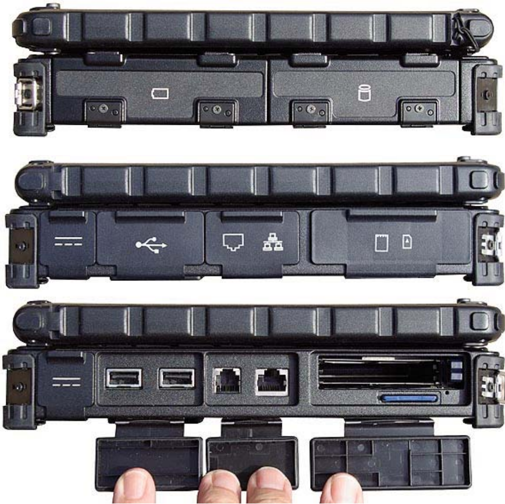
Top: Battery and hard disk compartment on the right side of the computer are sealed and secured. Bottom: Most ports and expansion slots along the left side of the V100 have individual, sealed protective covers.
