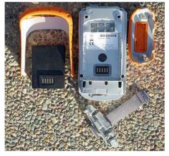
tic/rubber elastomer overmold by simply undoing a grand total of six screws and you find underneath an entirely more serious looking piece of equipment.
