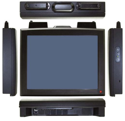
which should be minimized. Desired processing power also depends on the choice of operating system. RMT decided to be very flexible here and make it so the Duros 1214 can run a range of operating systems, beginning with very lean ones such as Windows XP Embedded or Linux, but also standard XP and even resource-intensive platforms like Windows Vista.
