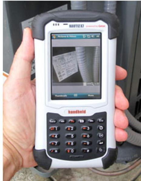
The picture above shows shows a Handheld Nautiz X7 (powered by Getac) ultra-rugged computer recording a spec label from an A/C unit. Integrated cameras are starting to become very useful.
