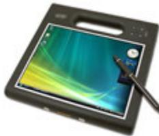
Optimal viewability both indoors and outdoors and from all angles have long been the Holy Grail of the mobile computing industry. Motion is getting several steps closer with the "View Anywhere" version of the Hydys AFFS+ display now used in its rugged F5 tablet. Motion also decided to upgrade to a Core 2 Duo chip instead of Atom, and that worked out quite well. [See review of the [updated Motion F5](#)]
