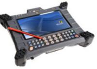
Measuring about 10 x 8 x 2 inches and weighing a bit over three pounds, the Atom Z530-powered DLI 8400 with its 7-inch WSVGA touchscreen and integrated magcard reader is significantly smaller and lighter than full-size rugged tablets but it is still large enough to serve as a full-function computer. In a detailed analysis, RuggedPCReview.com found the DLI 8400 a very competent and highly configurable ultra-mobile tablet
