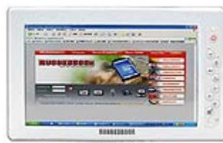
We've been seeing a move to ever greater ruggedness and better sealing in vertical market products where modest ruggedness used to be considered good enough. The latest version of Samwell's MCA9 medical/clinical tablet now carries IP65 sealing and can handle more abuse, in part due to a switch to solid state storage.
