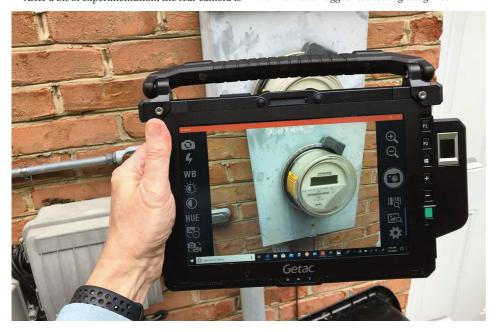
The UX10's IP65 rating indicates total protection against dust, and protection against low pressure water jets from all directions.
